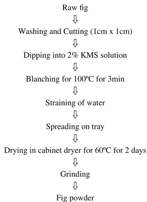
The samples were then dehydrated by using a cabinet dryer. Drying was carried out at 60°C for 24 hours for fig (Piga *et al.* 2004). The dried pieces were grounded by using a mixer grinder (Panasonic MX-AC555). Grinding was carried out at medium speed for 5 min. The ground powder was sieved using mesh containing a 20mm pore size. The diameter of the pore. Finally, fine powder was produced.
