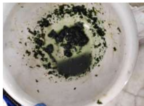
Figure 2. Diphenylamine test for the detection of nitrate in German grass sample. The content is after incubating processed grass samples with diphenylamine reagents.
